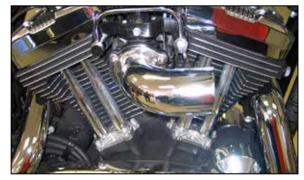
10. Install the K&N<sup>®</sup> intake tube onto the throttle body while attaching the vent hose to the vent tube and secure with the provided hardware. **NOTE: Apply one drop of the provided thread** locker to the K&N<sup>®</sup> intake tube mounting bolts, adjust the vent tube and intake tube/throttle body for best fit, and tighten the mounting bolts.
