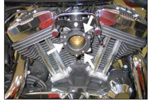
8. Install the K&N<sup>®</sup> intake tube adapter onto the throttle body using the provided hardware. NOTE: Apply one drop of the provided thread locker to the three tube adapter mounting bolts.
