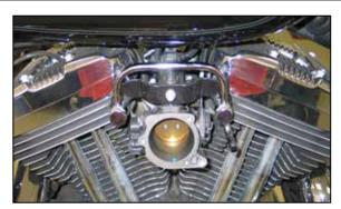
7. Install the K&N<sup>®</sup> crankcase breather tube onto the vehicle using the provided hardware. **NOTE: Do not completely tighten the breather bolts at this time.**
