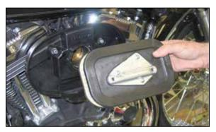
4. Remove the air filter as shown.
