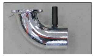
9. Cut the provided crankcase vent hose to a length of 1.75" and install onto the K&N $^{\odot}$  intake tube as shown.
