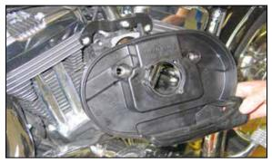
6. Remove the air filter base as shown. NOTE: K&N Engineering, Inc. recommends that customers do not discard the factory air intake components.
