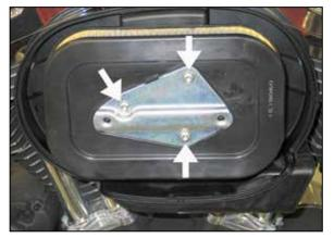
3.Remove the three air filter mounting bolts shown.
