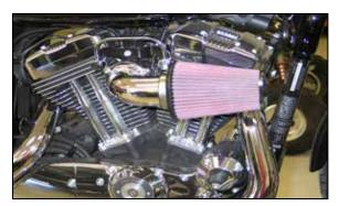
11. Install the K&N<sup>®</sup> air filter onto the K&N<sup>®</sup> intake tube and secure with the provided hose clamp. A black hose clamp is being supplied with kit. This clamp is intended to clamp the filter to the intake tube.
